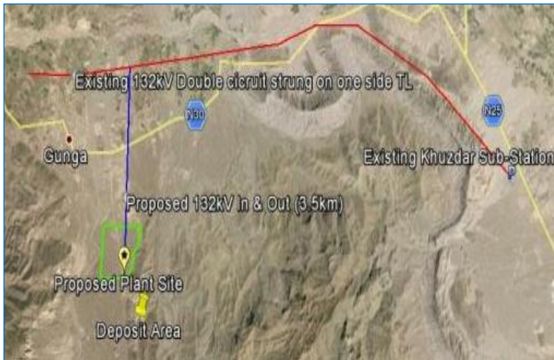
Figure 2.8: Proposed Transmission Line Scheme
