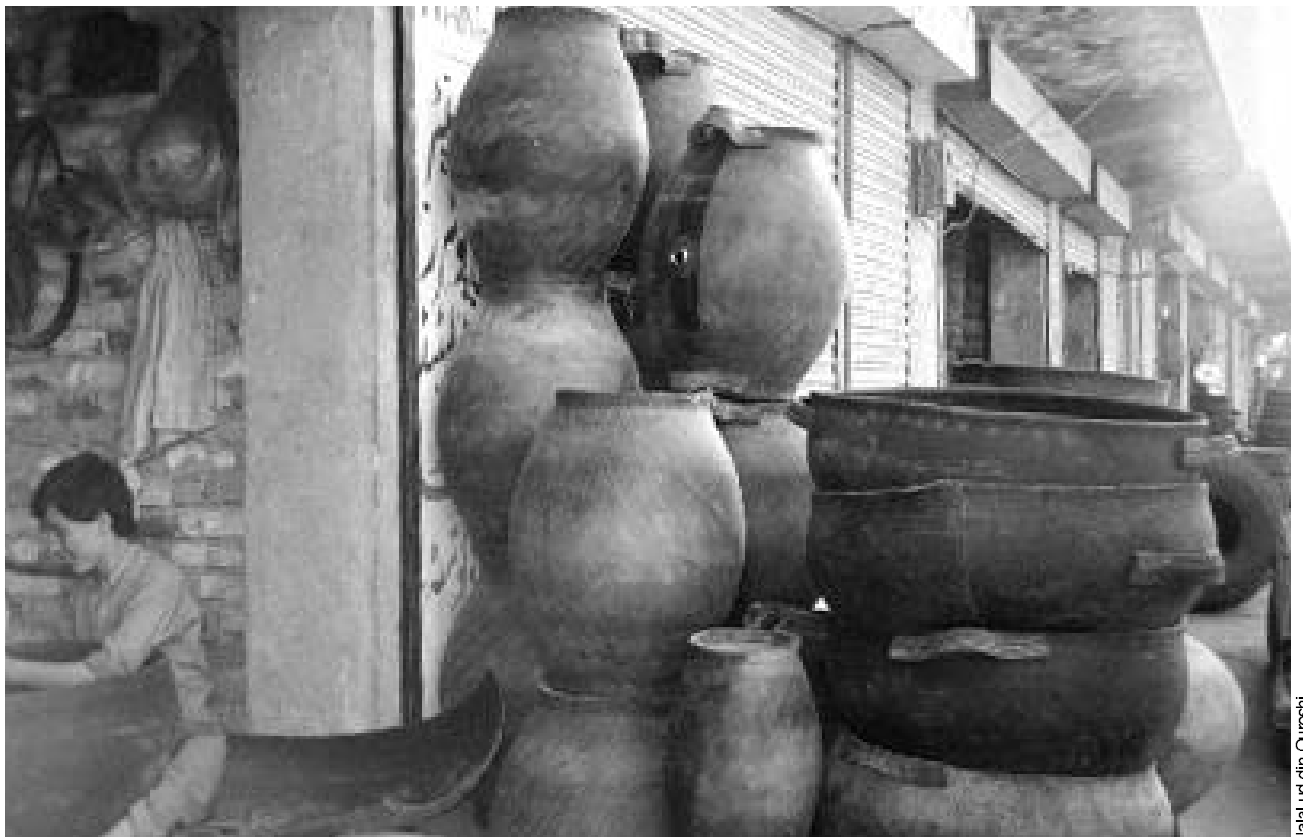
Ingenuity at work: water containers made from recycled tyres are in common use in Balochistan.
